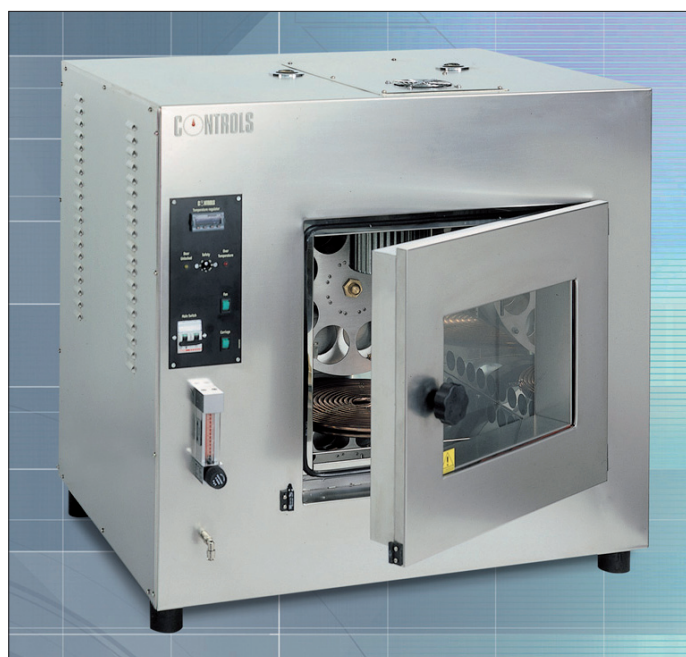
Figure 12 - The RTFOT (Rolling Thin Film Oven Test) equipment - EN 12607-1
