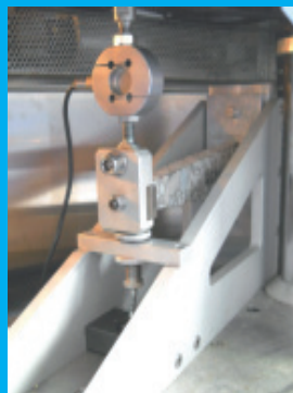
Figure 5 - The test accessory. For Stiffness by indirect tensile test UNI EN 12697:26 - Annex C
