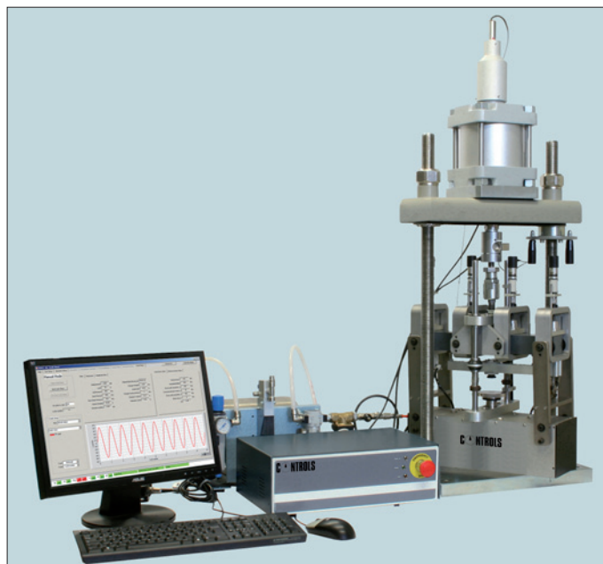
Figure 1 - Dynamic tests: set-up for the four-point bending fatigue test (Standard UNI EN 12697:24 - Annex D)
