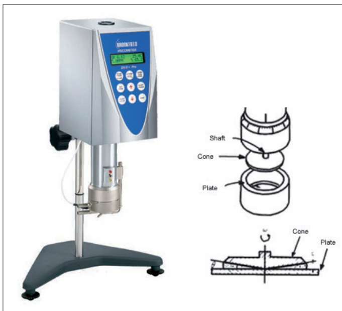
Figure 9 - The cone and plate viscometer (with reference to EN 13702 (GARDCO - Brookfield))
