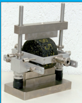
Figure 4 - The test accessory 2-point bending stiffness. EN 12697 - Annex A
