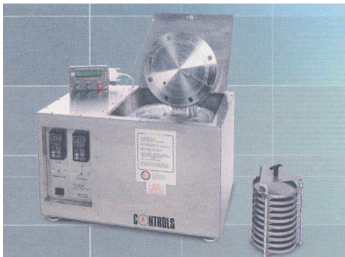
Figure 11 - The PAV, paving long-term ageing test (according to UNI EN 14769)
