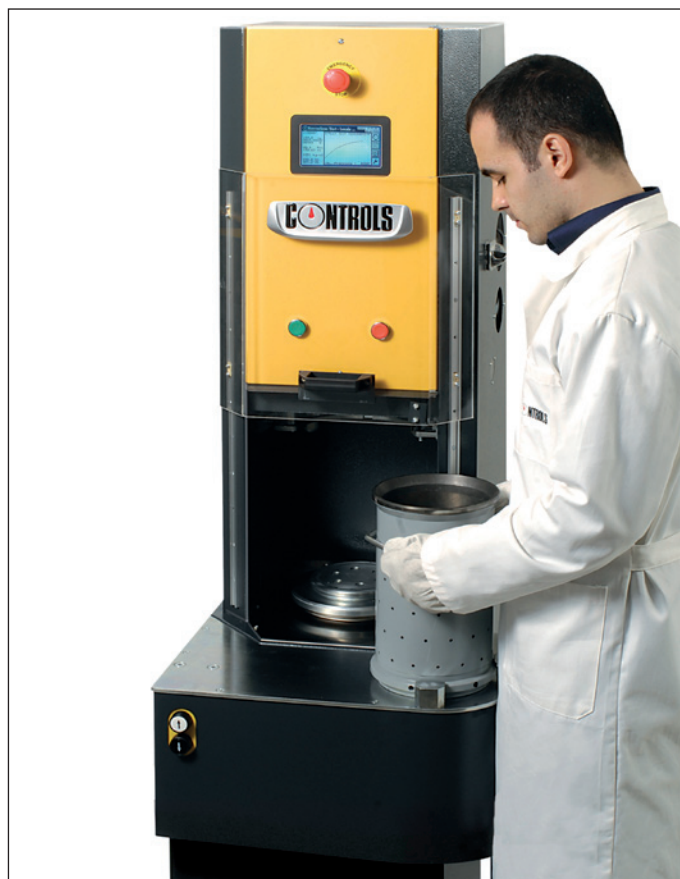
Figure 13 The gyratory compactor (according to EN 12697:31)
